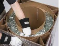
Remove the 2 crescent shaped cardboard inserts. Secure the butt end of the wire to the side of the box in preparation of the next step. Redistribute the gems on top of the wire.
