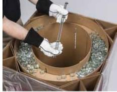
Cut rubber band from the support bar. Collapse and remove tie down bar by pulling each side towards the middle.
