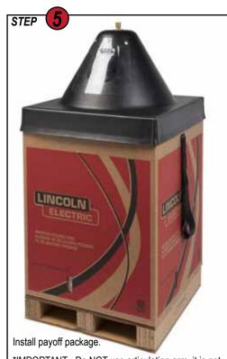
\*IMPORTANT - Do NOT use articulating arm, it is not designed to accommodate an inner core.
